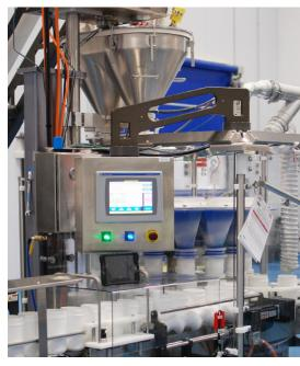
changing out the hoppers or augers for the different container sizes associated with this filler."
